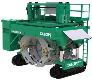
The Talon <sup>™</sup> 2000 — McElroy's biggest machine to date — brings a revolutionary new way to fuse large-diameter, thermoplastic pipe that is in growing demand to replace aging infrastructures and increase capacity for a variety of today's applications
